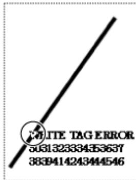
When using a small-size tag (about the size of P30 X W40 mm (P1.18" X W1.57"), for example) or not enough for setting margin, the slash and error message are printed overlap on each other. The overlapped area are inverse from black to white. There is no dump printing.
