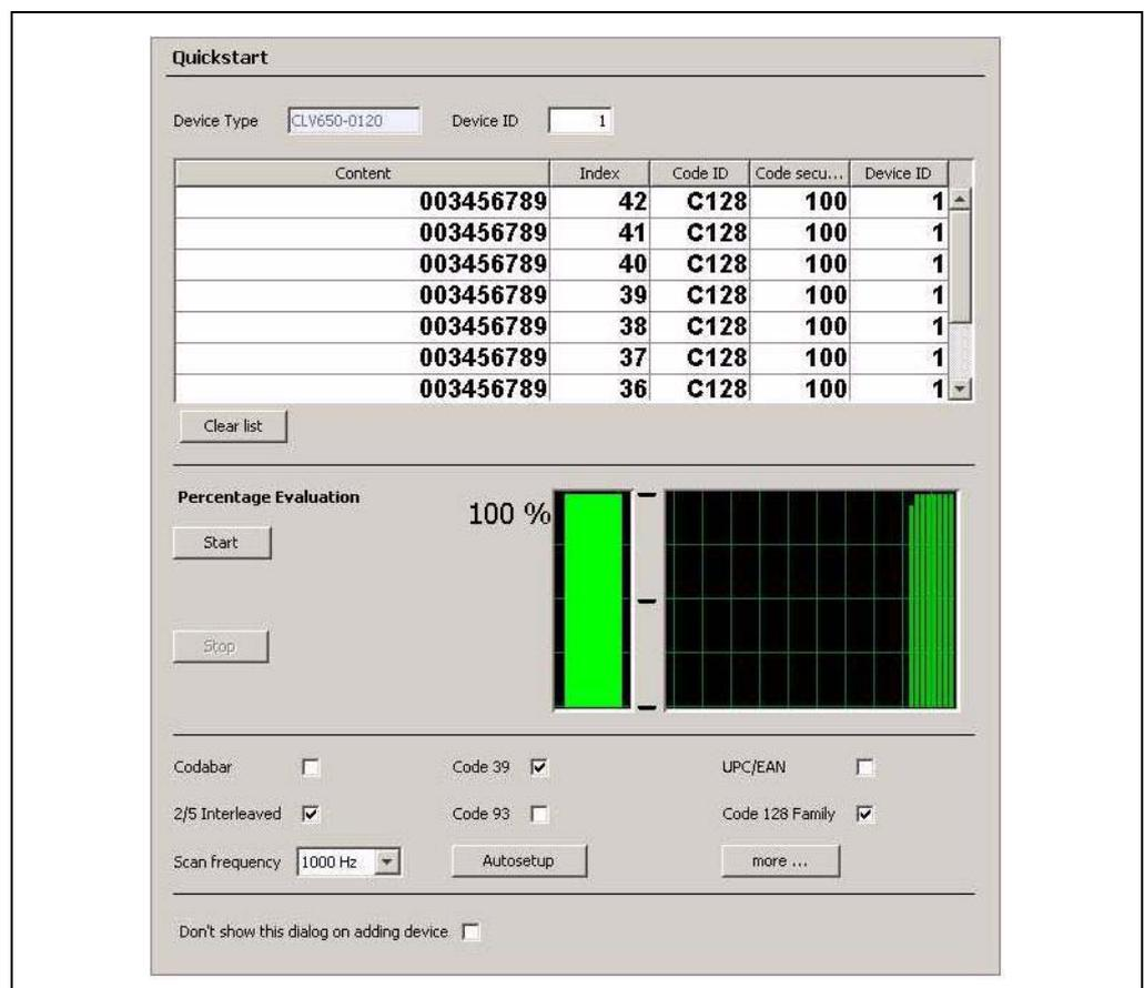
Fig. 3-1: Quickstart register tab of SOPAS-ET configuration software
