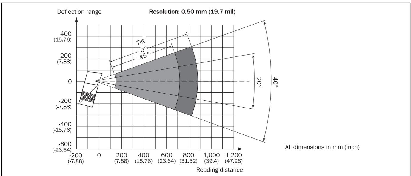
Fig. 10-19: CLV651: Deflection range as a function of the reading distance, deflection angle and resolution of 0.5 mm (19.7 mil)
