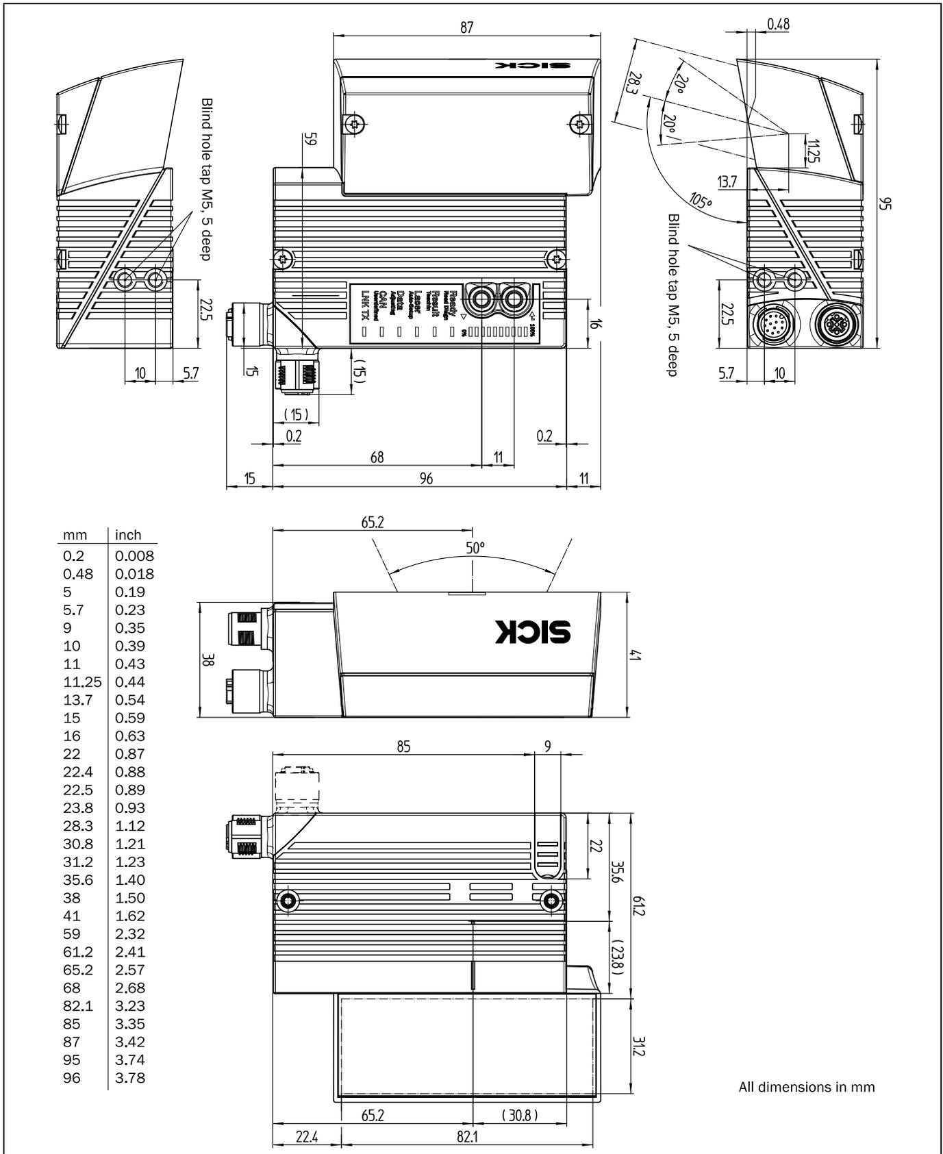
Fig. 10-23: Ethernet version: Dimensions of the bar code scanner with oscillating mirror (CLV65x-6120)
