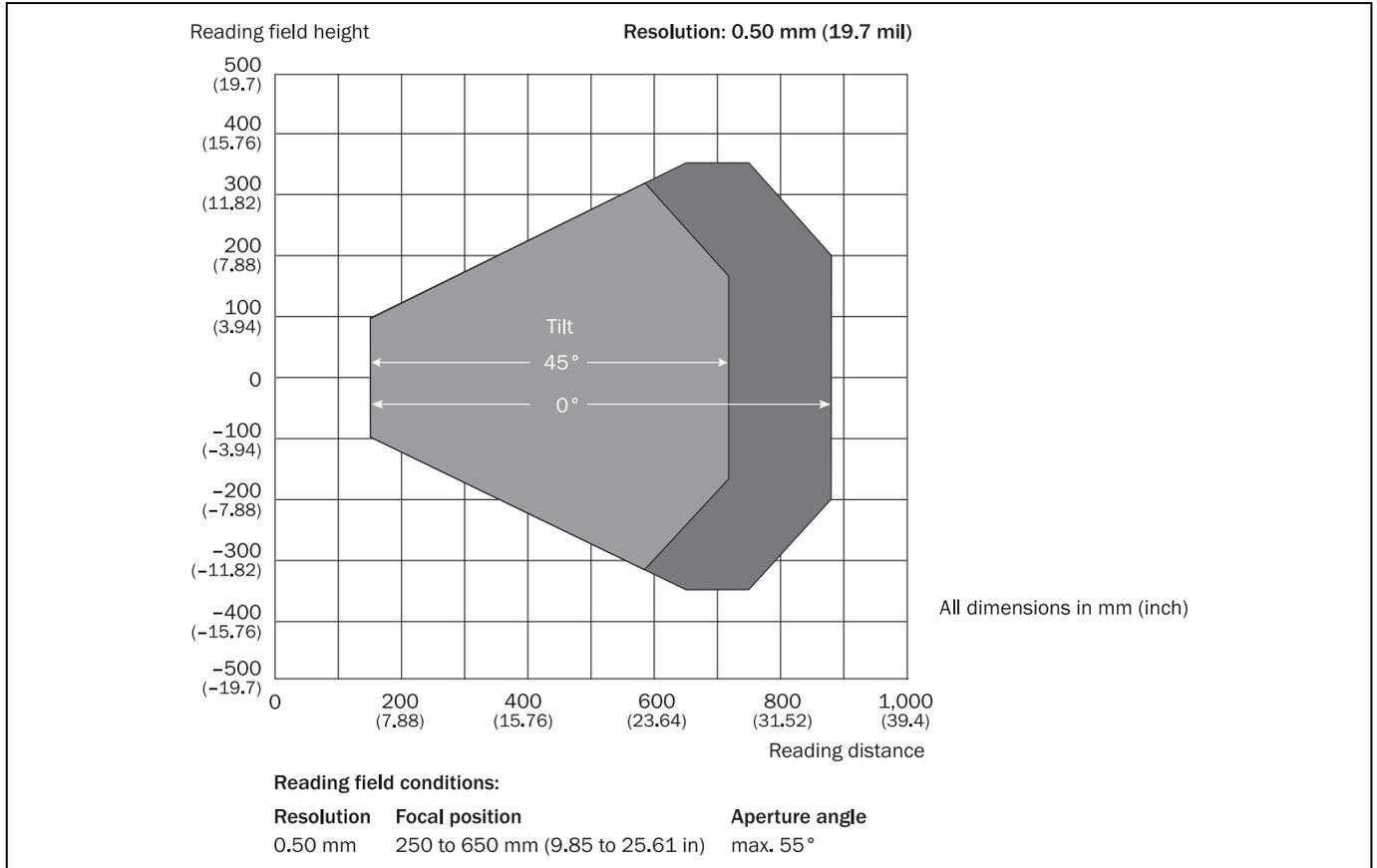
Fig. 10-15: Depth of field ranges of the CLV651 line scanner with oscillating mirror (side reading window): Resolution 0.5 mm (19.7 mil) and inclination angle 0°/45°
