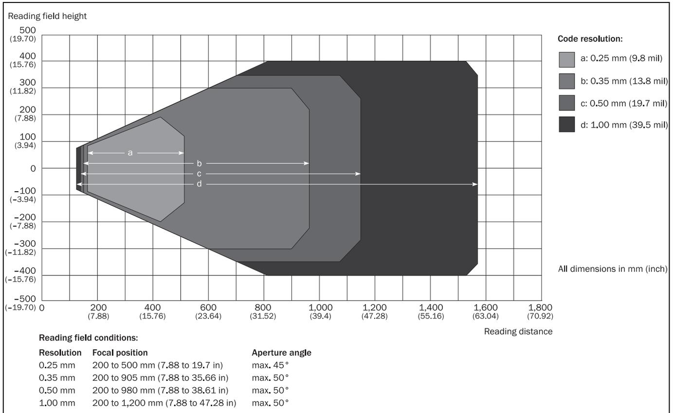
Fig. 10-7: Depth of field ranges of the CLV650 line scanner with oscillating mirror (side reading window): Resolutions 0.25 mm (9.8 mil), 0.35 mm (13.8 mil), 0.5 mm (19.7 mil) and 1.0 mm (39.4 mil)
