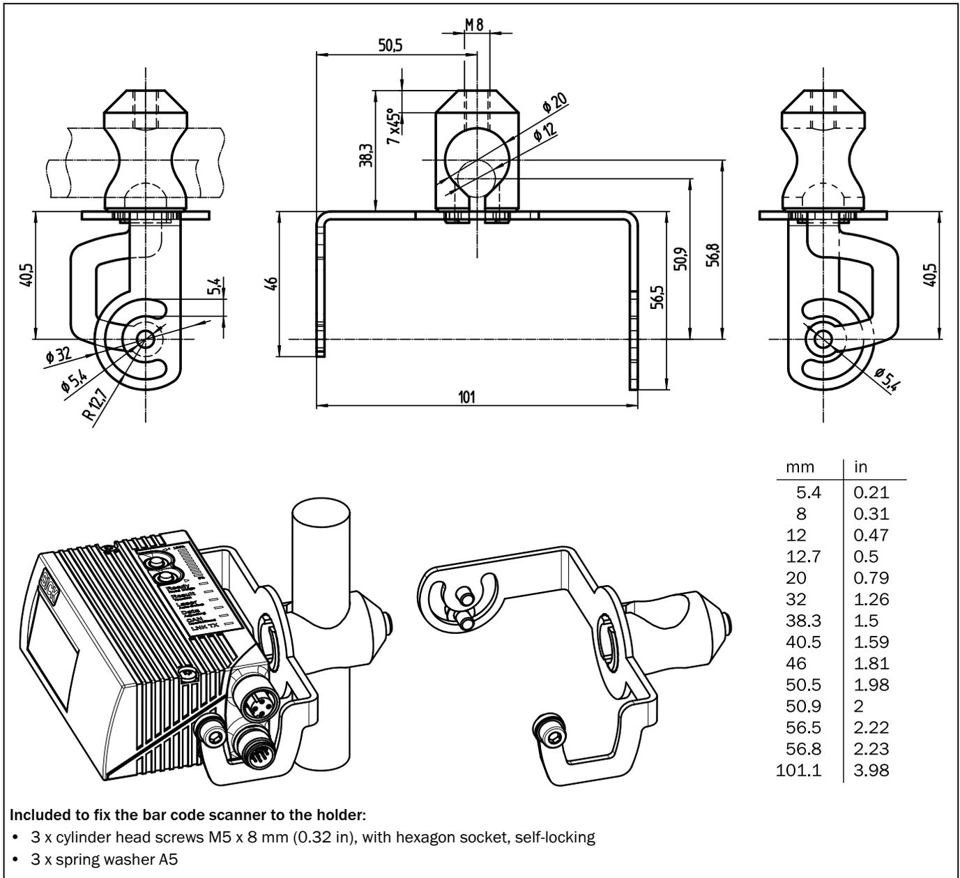
Fig. 11-4: Dimensions of the round rod holder no. 2042801
