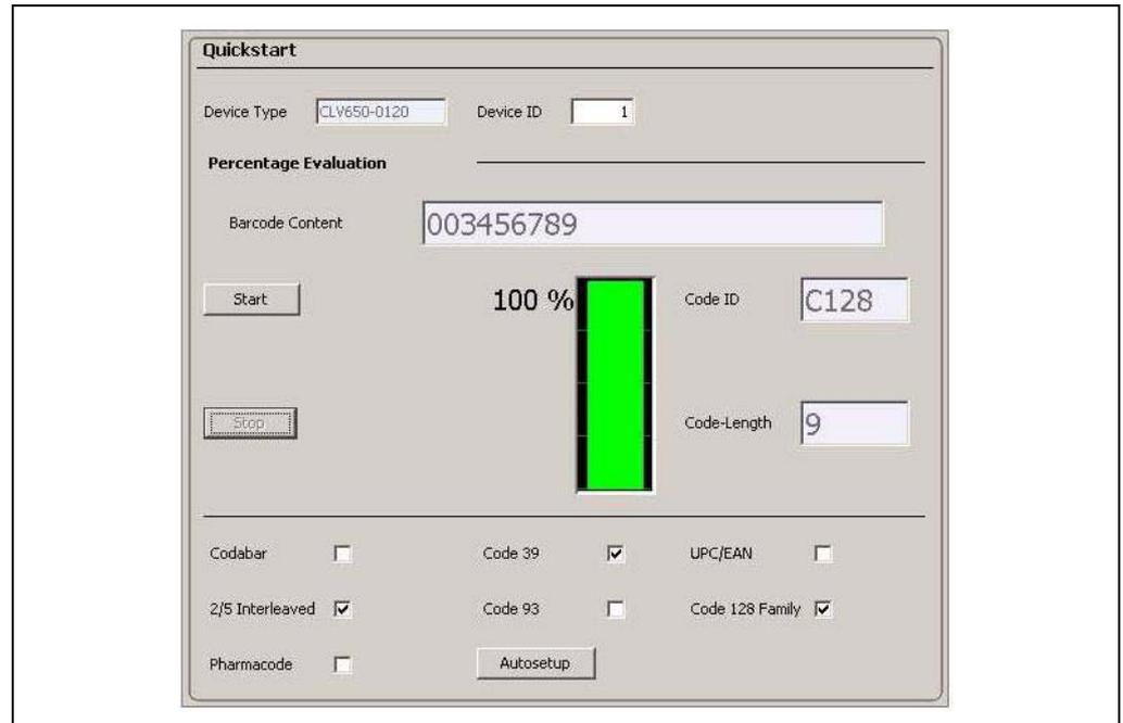
Fig. 3-2: Quickstart register tab in Single Device Mode
