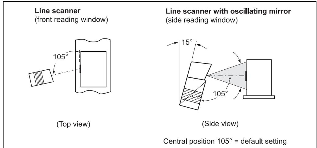
Fig. 5-6: Avoiding surface reflection using the line scanner as an example: Angle between emitting light and bar code (tilted away from the plumb line)
