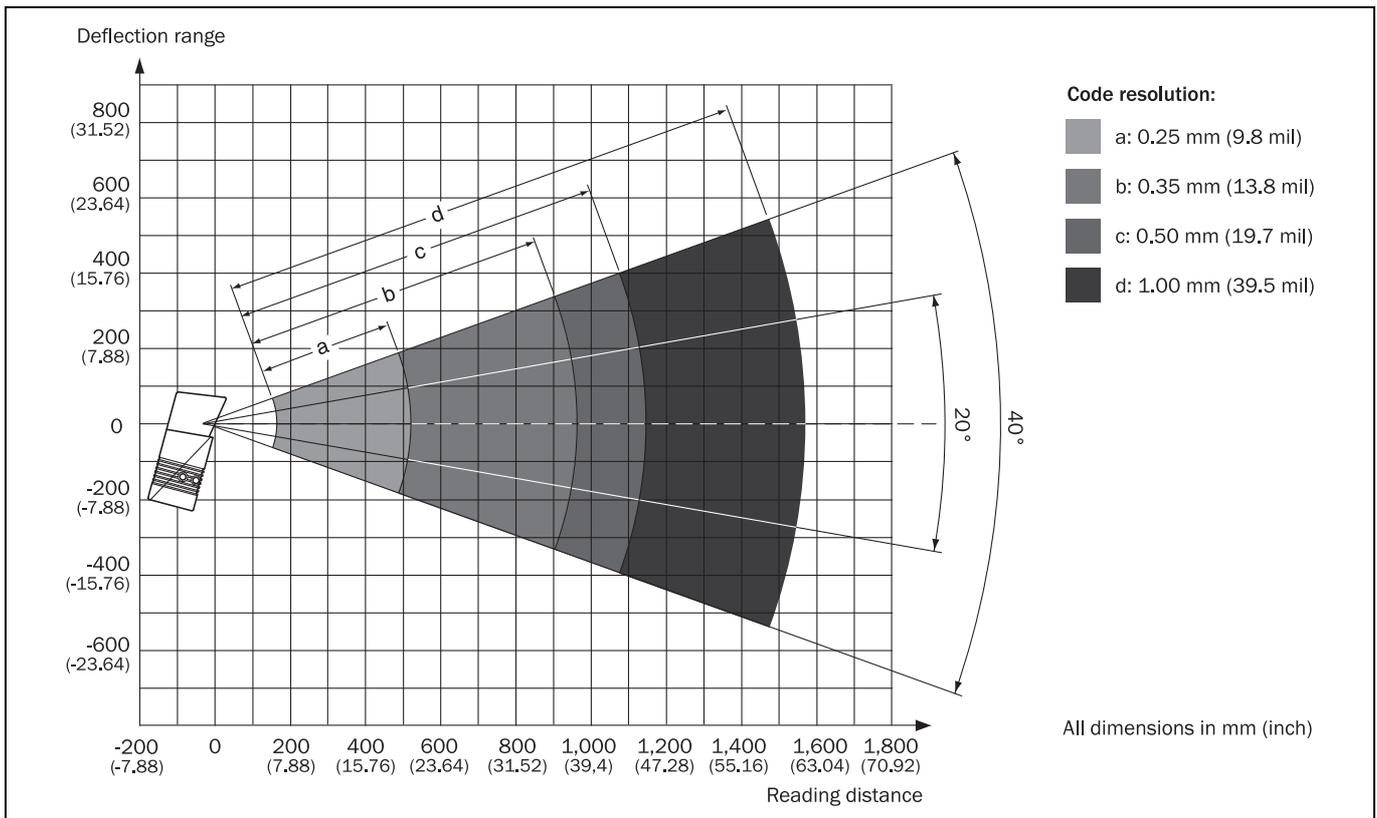
Fig. 10-18: CLV650: Deflection range as a function of the reading distance, deflection angle and resolution
