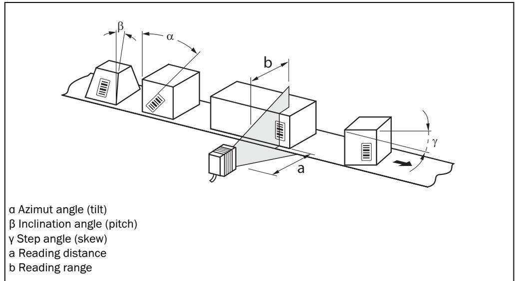
Fig. 5-5: Line scanner: Reading angles that occur between the scanning line and bar code
