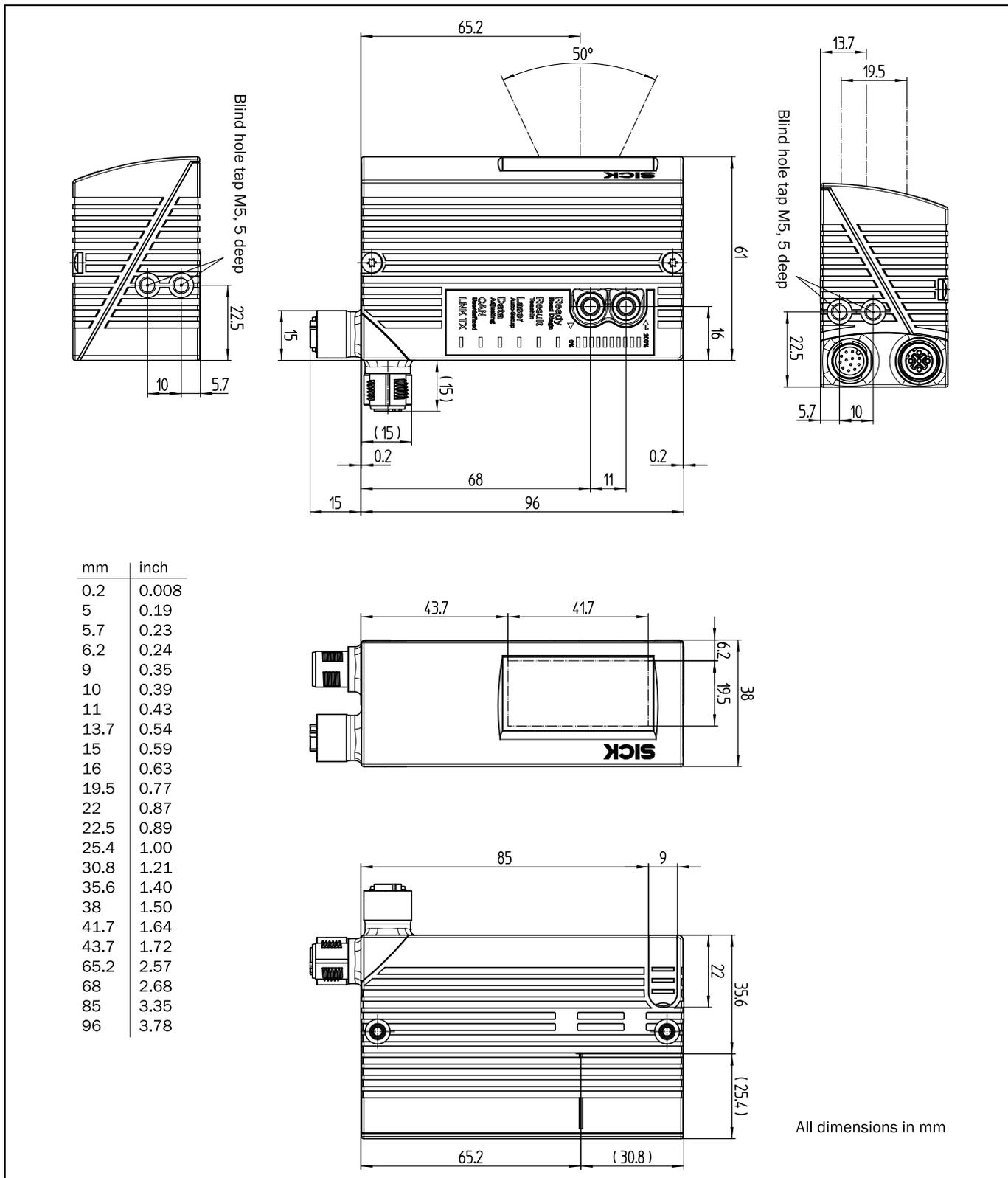
Fig. 10-22: Ethernet version: Dimensions of bar code scanners with front reading window (CLV65x-0120)
