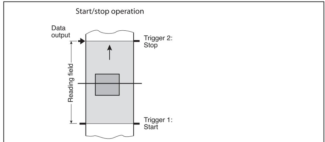
Fig. 4-7: Reading operation mode for the CLV65x bar code scanner in stand-alone operation
