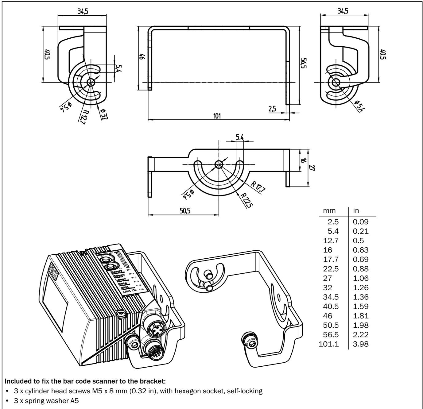
Fig. 11-3: Dimensions of the fixing bracket no. 2042800
