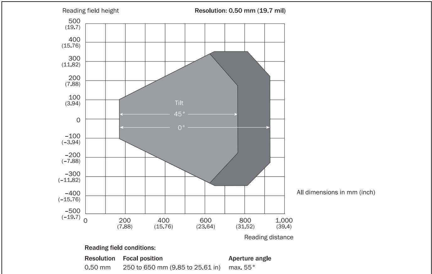
Fig. 10-12: Depth of field ranges of the CLV651 line scanner with front reading window: Resolution 0.5 mm (19.7 mil) and inclination angle 0°/45°
