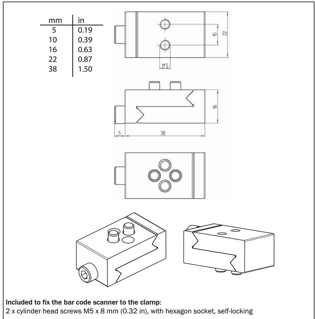
Fig. 11-2: Dimensions of the quick release clamp no. 2025526
