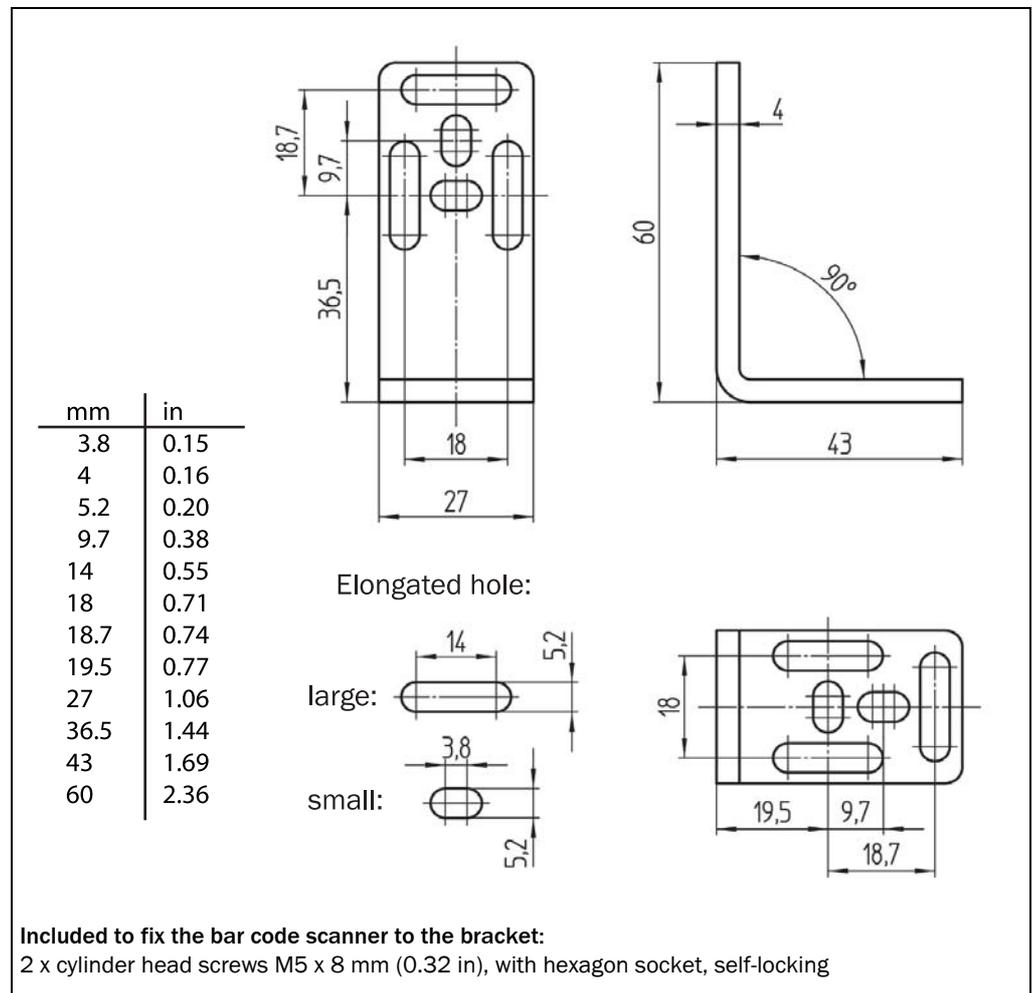
Fig. 11-1: Dimensions of the fixing bracket no. 2020410
