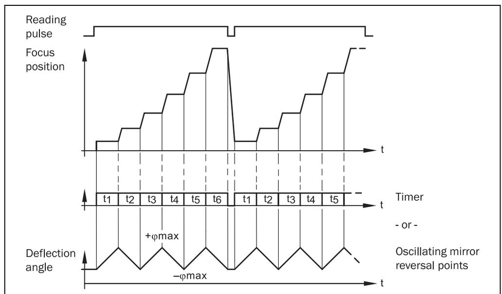
Fig. 4-6: Oscillating mirror CLV65x: Example of focal position control in search run, here with 6 focus positions
