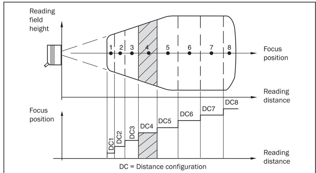
Fig. 4-5: Switching the focus for CLV65x: Division of the entire reading area in distance configurations
