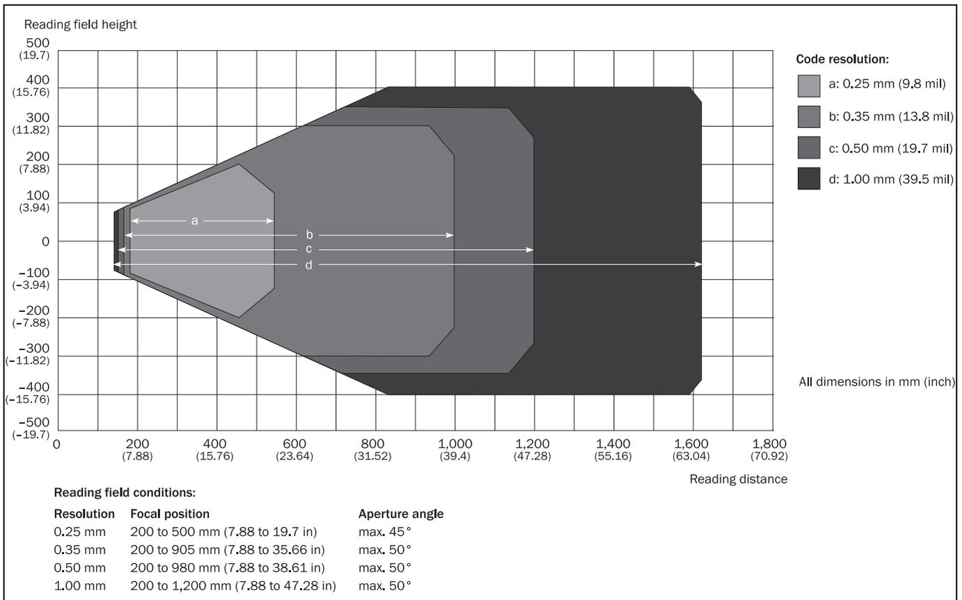
Fig. 10-2: Depth of field ranges of the CLV650 line scanner with front reading window:
