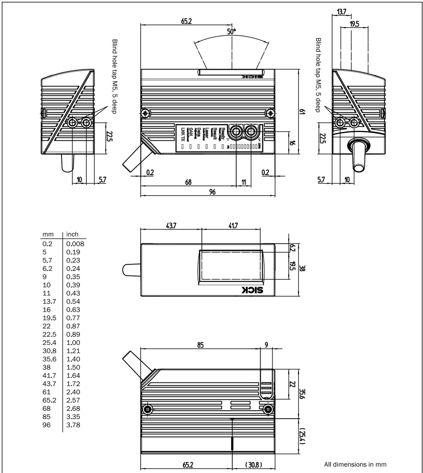
Fig. 10-20: Standard version: Dimensions of bar code scanners with front reading window (CLV65x-0000)
