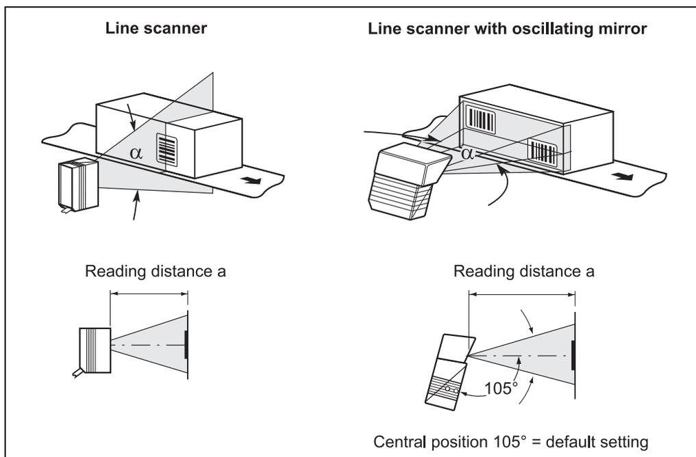
Fig. 5-4: Definition of the reading distance a and the aperture angle  $\alpha$
