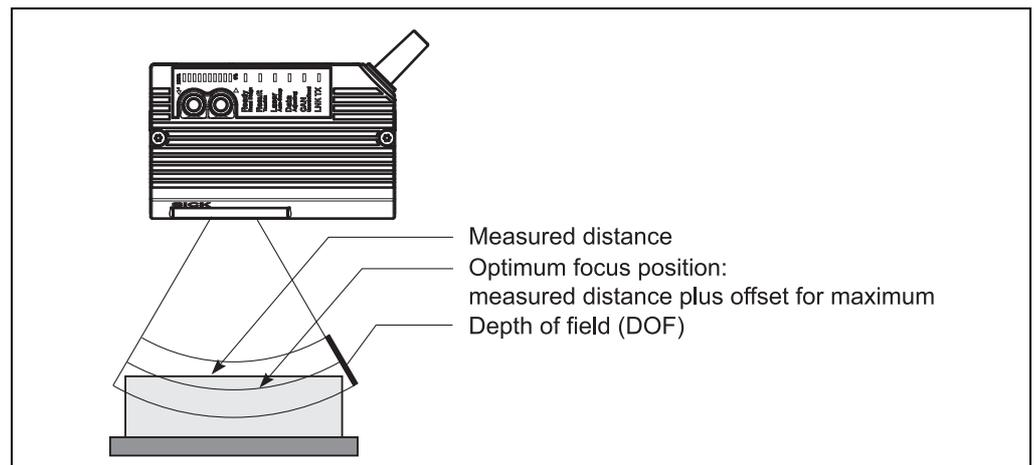
Fig. 4-4: Optimization of the depth of field for the object
