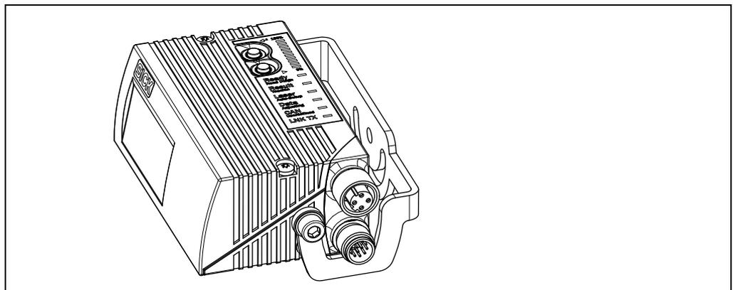
Fig. 5-1: Example: Fixing the bar code scanner with the bracket no. 2042800
