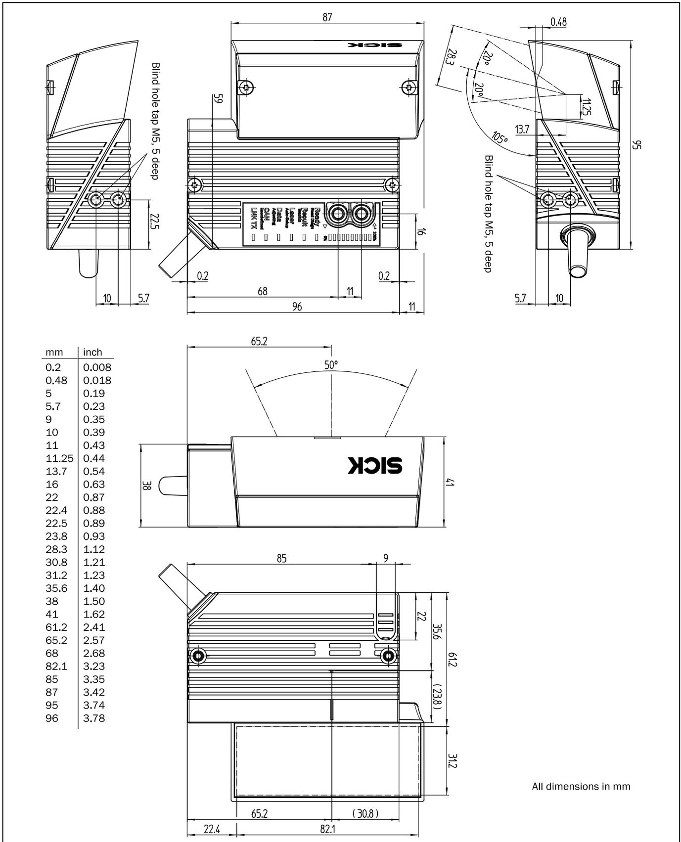
Fig. 10-21: Standard version: Dimensions of the bar code scanner with oscillating mirror (CLV65x-6000)
